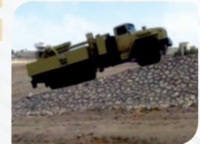
Egypt demonstrated the new self-propelled howitzer by the integration of the howitzer 122mm D-30, mounted on a modified truck chassis Ural-4320-1911-30 with the wheel formula 6X6., The truck features YAMZ-238M2 (240 hp) diesel engine.
